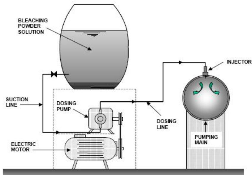
Figure - 5: Bleaching Powder Dosing Arrangement
