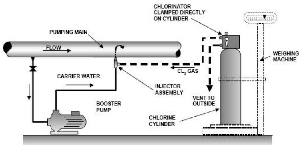
Figure - 6: Gas Chlorination Arrangement
