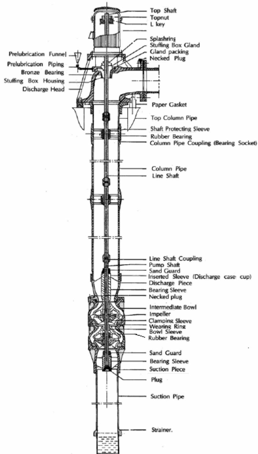
Figure – 2: Turbine Pump
